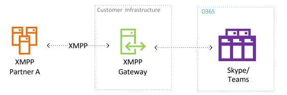
The server communicates with O365 components using O365 APIs and SIP via the public network, and via server-server XMPP/TLS with a remote XMPP domain.
