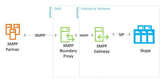
MindLink are investigating development of such a proxy alongside the main gateway component, given customer need. This proxy would enforce protocol-level authentication and validation, before any traffic reaches the internal network.
