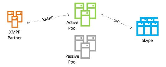
Failover of external XMPP connections is made by changing external DNS records and network configuration. Failover of internal SIP connectivity is made by the standard trusted application failover process.
