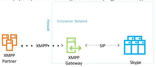
The server will communicate via SIP/TLS with the Skype for Business frontend pools over the internal network, and via server-server XMPP/TLS with remote XMPP domains.
